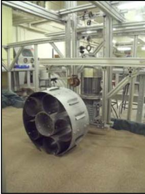
Figure 13 Single wheel testbed
