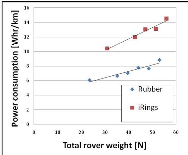
Figure 24 Power consumption for 5in wheels
