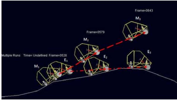
Figure 10 ADAMS model of a rover under both terrestrial and lunar gravity [12]
