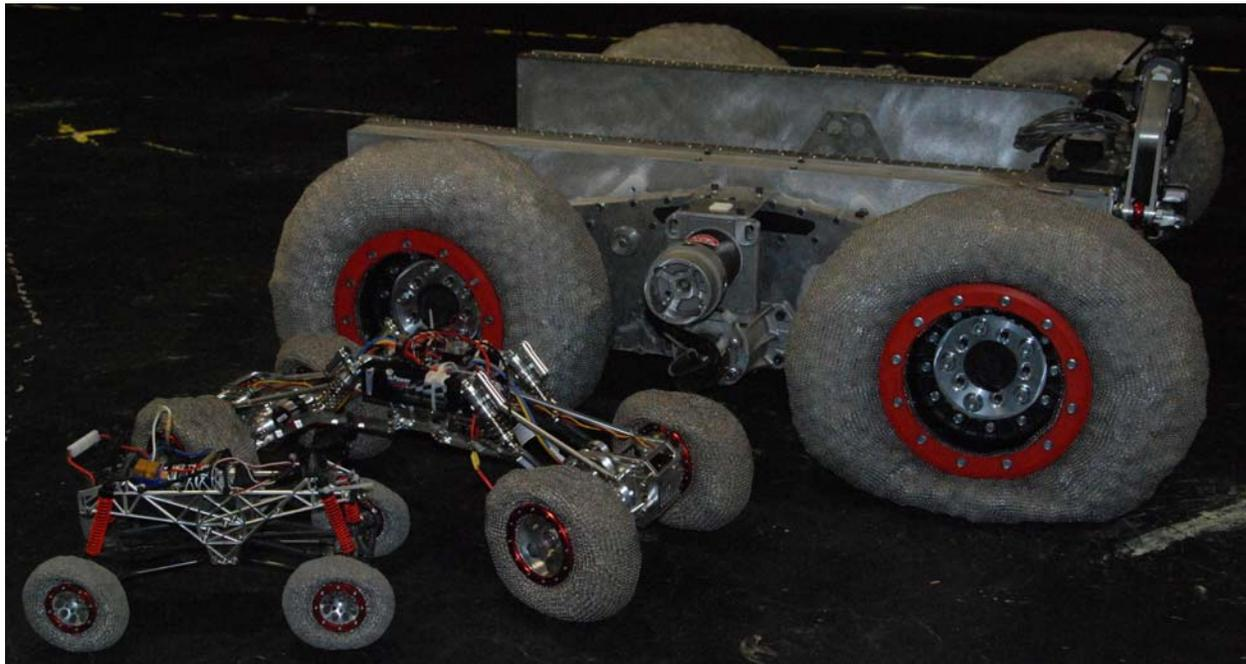
Figure 25 The suite of “iRings” prototype wheels – 5inch, 8 inch and 22 inch diameter
