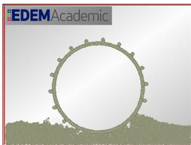
*Figure 7 3D DEM model of wheel thin section on lunar regolith*
