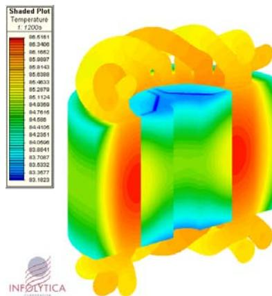
Figure 12 Simulation of temperature gradients induced by electromagnetic field in an brushless DC motor
