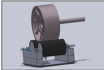
Figure 14 Drawing of twin roll wheel dyno [13]
