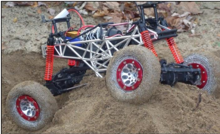
*Figure 21 5" iRings wheels on reduced scale rover*
