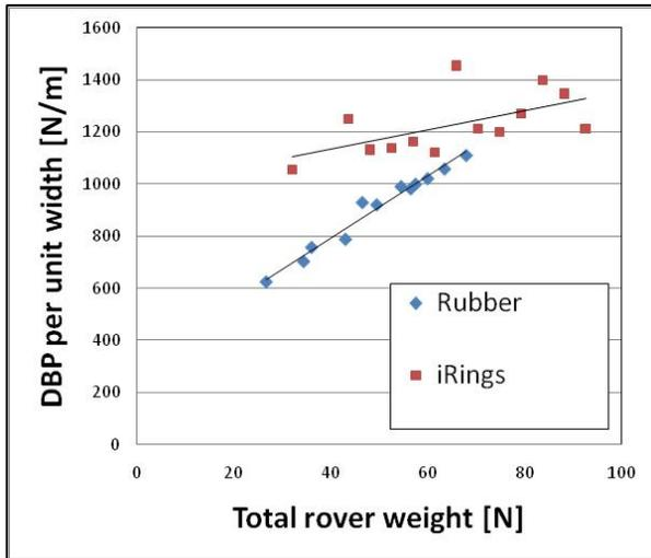
Figure 23 Ratio of drawbar pull / unit wheel width for 100% slip
