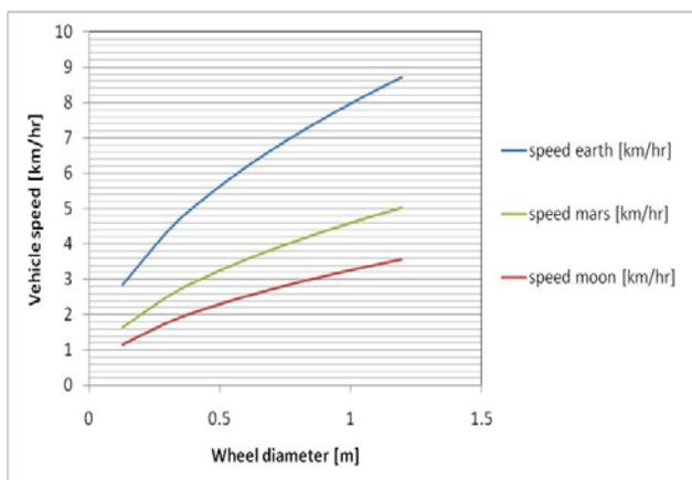
Figure 20 Critical driving speeds for iRings wheel with respect to wheel diameter
